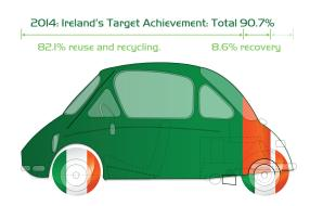
The targets are a mixture of reuse, recycling, and recovery of car (M1) and van (N1) ELVs. From 2015, the waste management of ELVs must achieve a two-fold target: 85% reuse and recycling, and 95% reuse, recycling and recovery. In essence, the difference between the two targets is the amount that may go to an incineration facility for energy recovery. This means that reuse and recycling is given priority.
